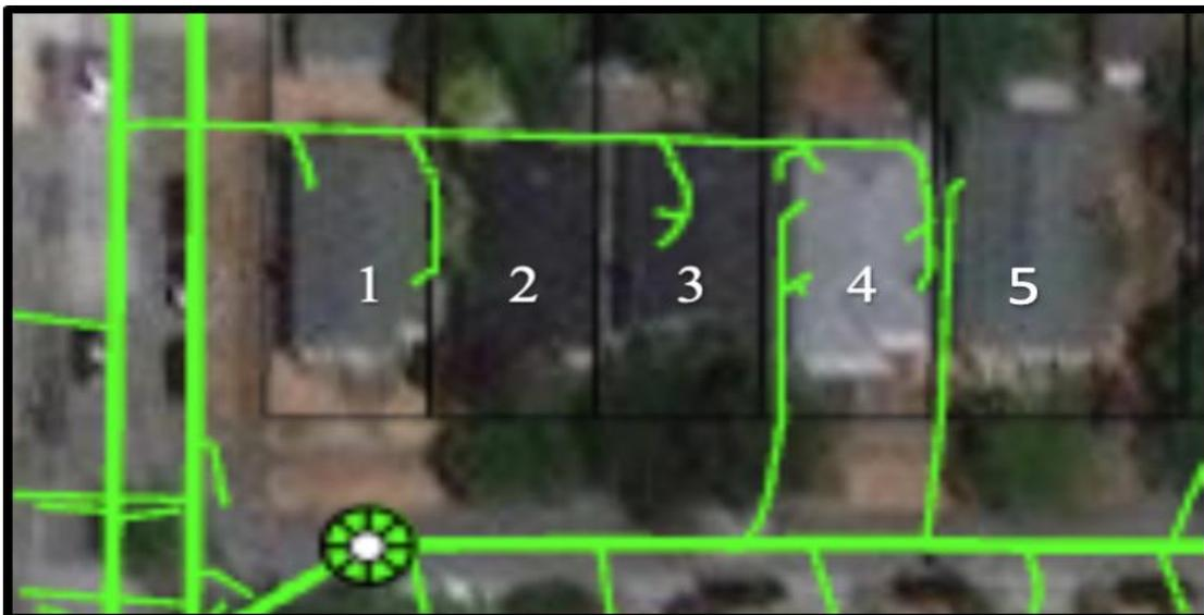
Figure 11: Note structure 4 is connected to 2 mainlines and has 3 additional structures on one lateral. Additionally, the need for good location accuracy of field locations is illustrated by the closeness of two laterals at the property line between 4 and 5.
