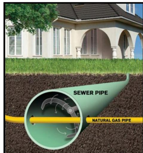
Figure 1: Graphic of sewer cleaning risk of a gas cross bore in sewer
